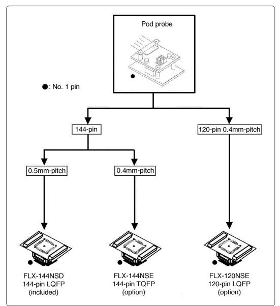
Figure 3.5 Connecting the target system
